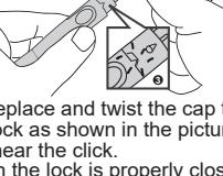
4. Replace and twist the cap to close the lock as shown in the picture until you hear the click. When the lock is properly closed lock indicator is in the extreme right position.
